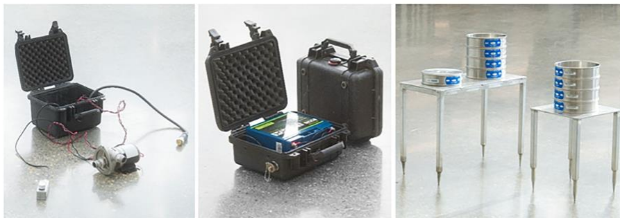
Fig. 2. High throughput microplastic sampling system components: centrifugal pump with electronics housed in a protective case (left), lithium iron phosphate battery housed in a protective case (center), cascading sieve stacks for samples and blanks with aluminum tables (right).
