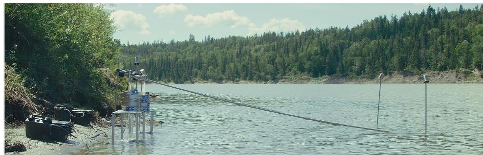
Fig. 4. Duplicate set-up of NAIT high throughput microplastic sampling system on the North Saskatchewan River.
