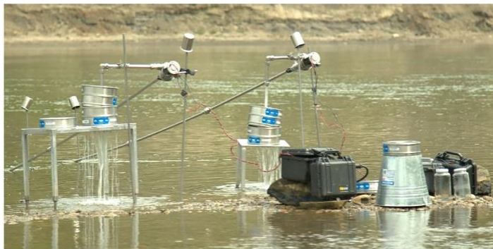
Fig. 3. Pumping river water in the field through a cascade sieve stack using 2 high throughput microplastic sampling system.
